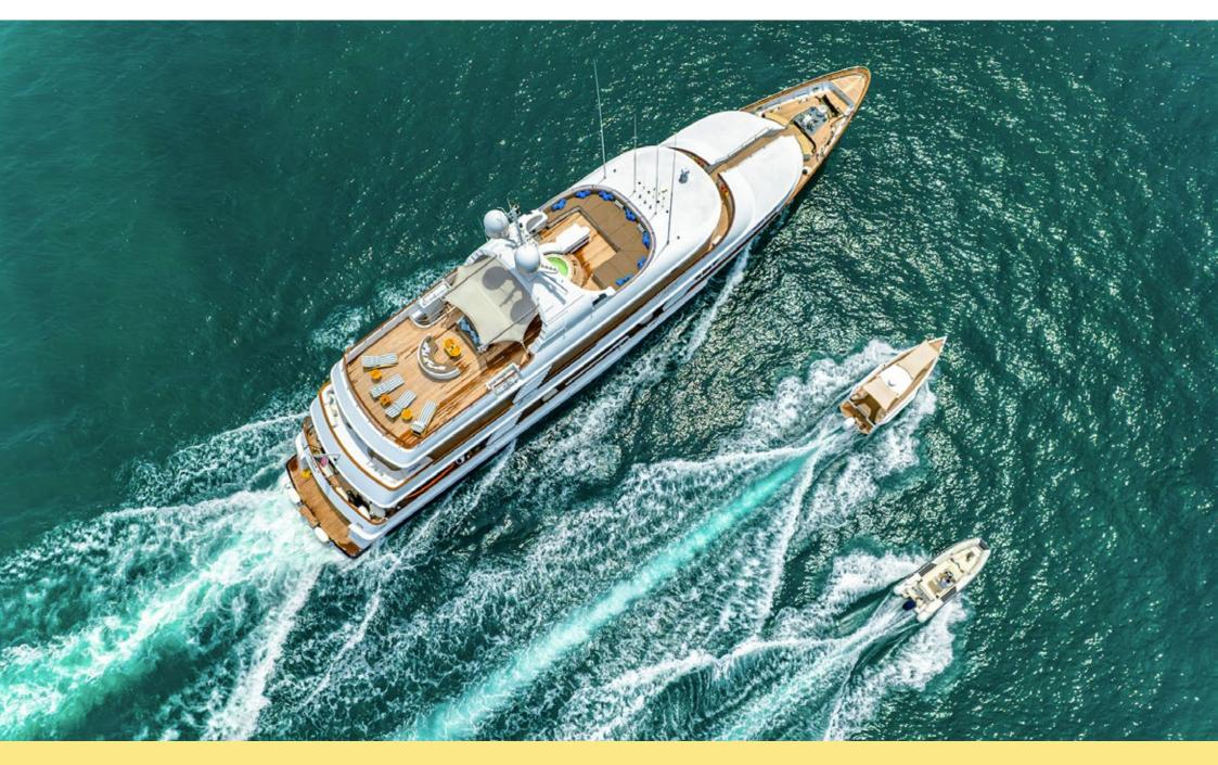
The boat was built by CRN in 1996, while her classic Italian-styled exterior is the work of exterior designer Paolo Scanu. The yacht was built in steel and aluminum and is RINA classed and MCA compliant. In 2015, the motor yacht completed a comprehensive two-year rebuild, which included teak decking, technical spaces, a full repaint of the exterior and more.
